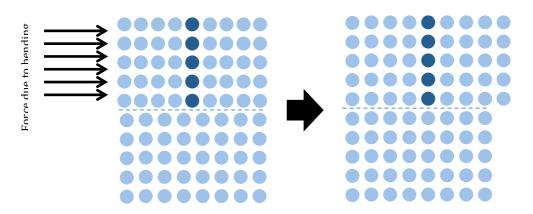
Motion of dislocation with increased force. Plans of atoms slide over one another to reach the edge
